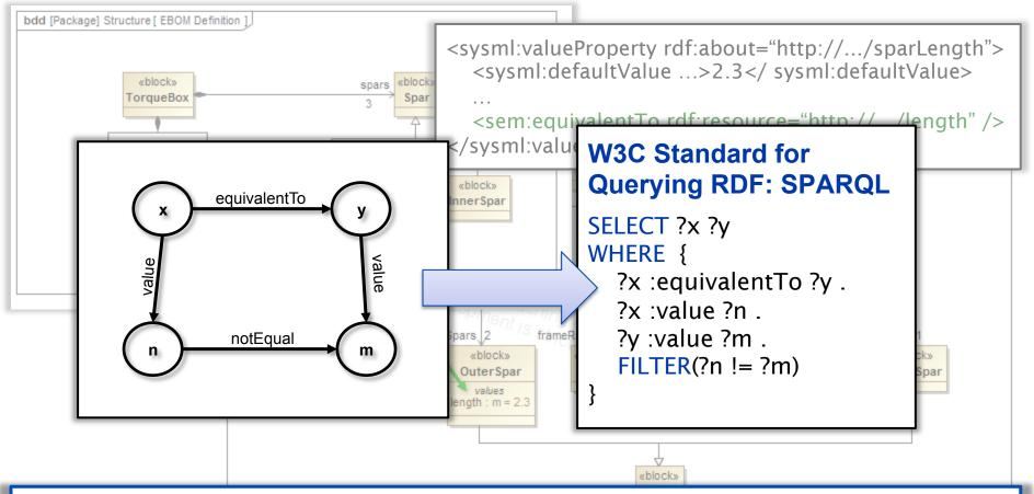
Inconsistency patterns (and, generally, inconsistency rules) are represented in a language such as SPARQL and executed using a corresponding engine
