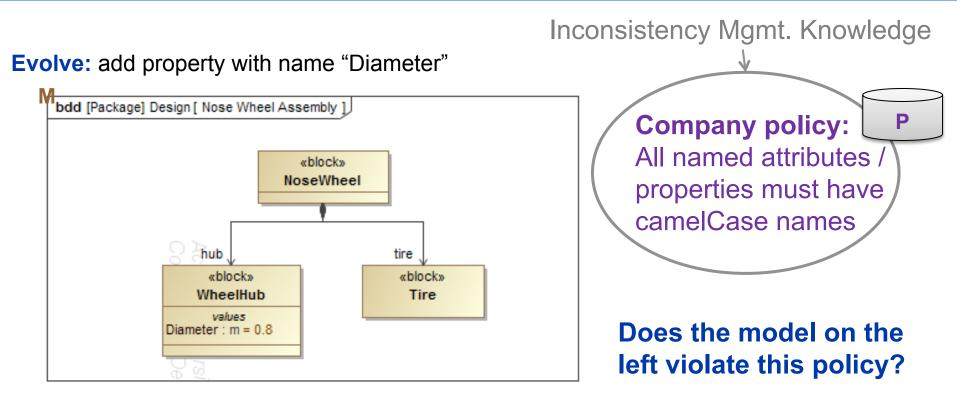
Check: the property's name is "Diameter" (M) ⇔ The property's name must be "diameter" (P)
