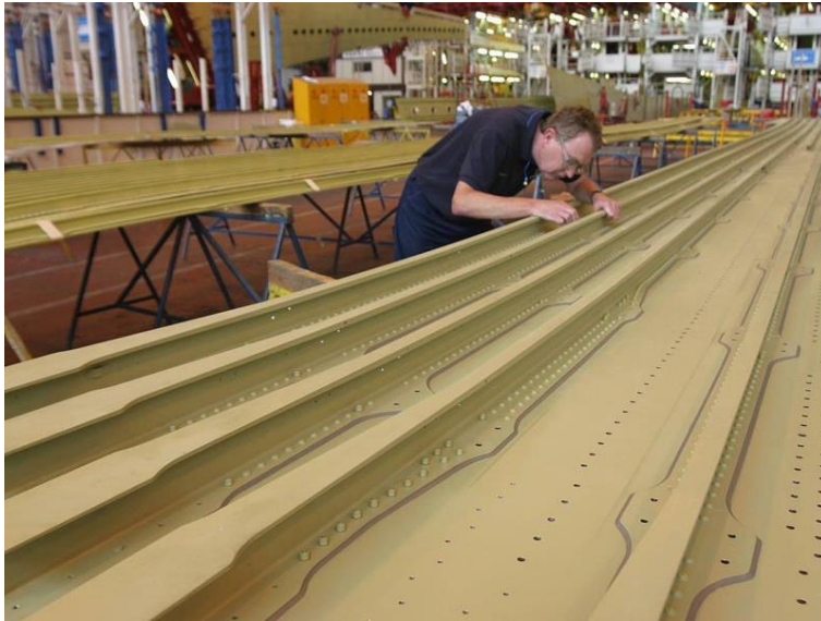
Example Bolted Aluminium Wing Skin
