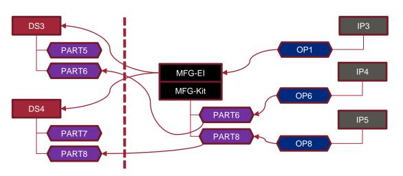
Typical use case: End item shipped from supplier with boxed kit for final assembly
