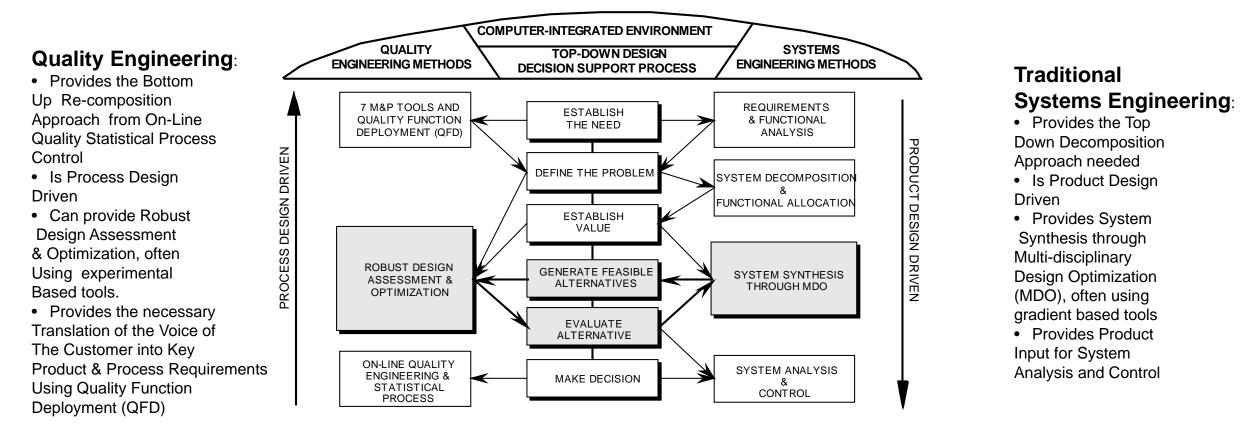
**Computer Integrated Environment Provides the Data Exchange as Indicated by Arrows**
