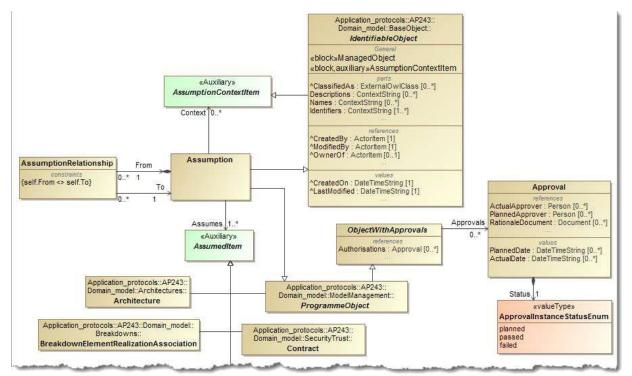
SysML block definition diagram for an application domain model
