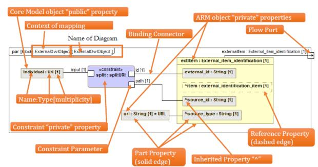
A parametric diagram mapping is "owned" by the source model Block object
